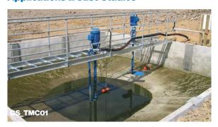
**CS\_TMC01**Extender pump and long shaft stirrer on fixed frame
